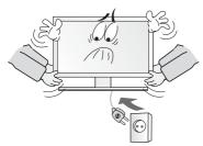
Before moving the product, ensure to switch off the power and unplug all the electrical cords and the external connection cords such as an antenna cable and other source connections, etc.
